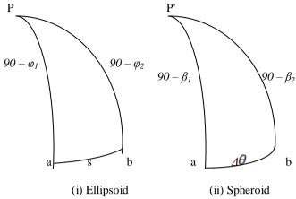
Figure (1): Ellipsoid and equivalent spheroid
